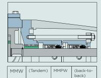
Double mechanical shaft seals, DIN 24960/EN 12756 - KU, in tandem or back-to-back, with productlubricated main bearing. Used where no leakage is allowed. Up to 16 bar differential pressure.
